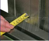
The minimum distance between the rear of the table and column. Depending upon available space it may be necessary to select a slim profile scale or mount on the front of the table.
