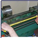
**STEP 4.** Measure between the mark and the edge of the carriage. This will give you the carriage travel.
