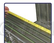
The overall length of table & gap between any table drains. To ensure the scale is easier to fit on the machine. Measure maximum length scale that can be fitted on each axis.
