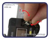
6. Insert replacement battery edge against side contact.
